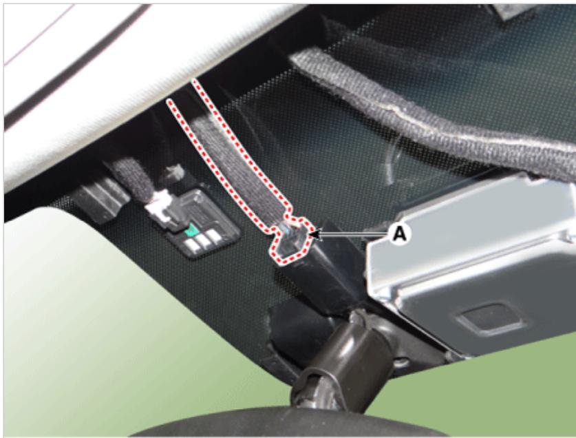
3. Remove the inside rearview mirror (A) by pulling it up in the direction of the arrow.
